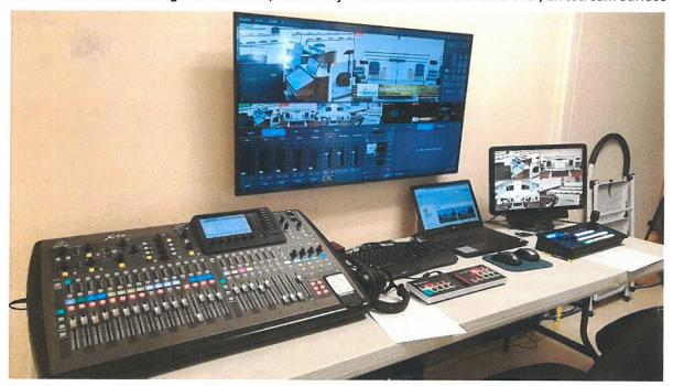
Go switcher panel, monitors, cables, USB audio interface, and a custom designed/built Intel i9/Windows 10 computer with sufficient capabilities to handle it all. The computer includes up to 6 SDI video inputs and 2 SDI video outputs. To date total expenditures for the project in 2020 are \$24,713.30 not including repairs/improvement to our network and internet connection following the lightning strike. Most, if not all the funds, came from designated gifts not from the general fund.
